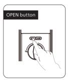
Double press the [OPEN] button within one second, and then push or pull the door to unlock the door.
