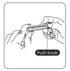
① Cut the mechanical key box and take out the key shell. Push the knob aside and reveal the key itself.
