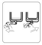
③ Rotate the key cell 180° downward so it can be parallel to the ground, then rotate it horizontally toward the lever to unlock the lock.
